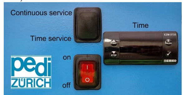
Switches for on/off and operation mode,
