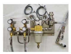
The central part of the breathing air supply from bottles is the pressure control station. It reduces the pressure of the compressed air cylinders, which can also be provided as a complete cylinder bundle, from up to 300 bar to 0 ... 16 bar. For monitoring and signaling of upstream and downstream pressure, the pressure control station has contact pressure gauges whose switching point can be selected individually.
