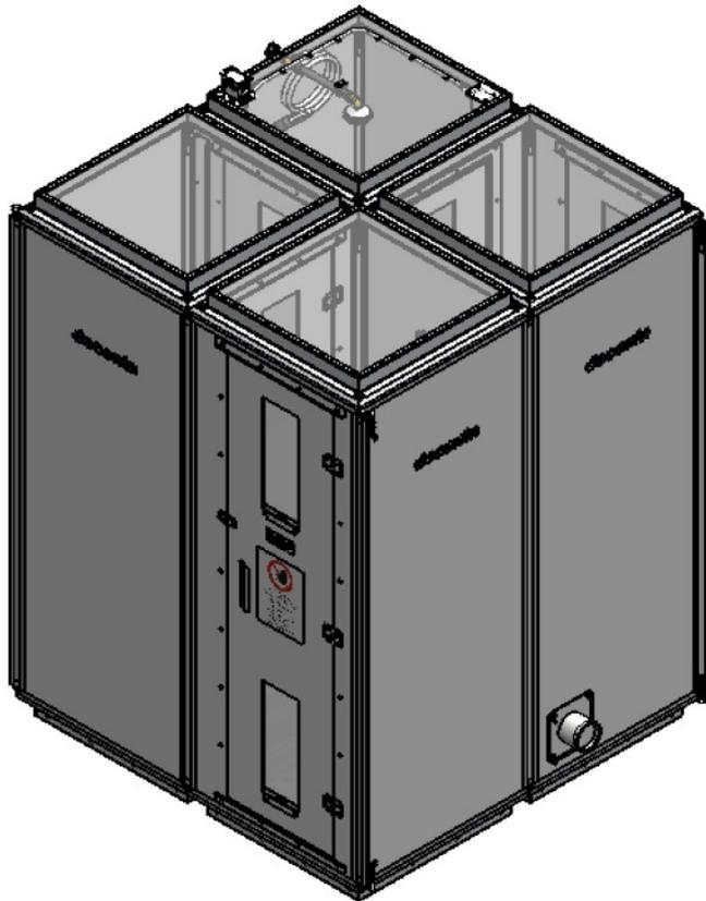
4 chambers, arranged in a square, with water shower in the 3rd chamber, without or with forced locking
